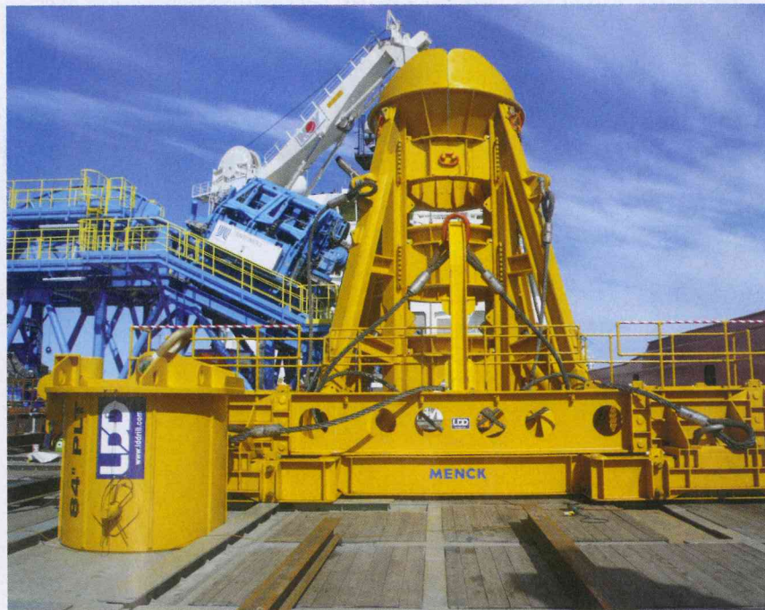
Fig. 4—Large Diameter Drilling Ltd. and Menck GmbH's StabFrame subsea pile-stabilizing template.
